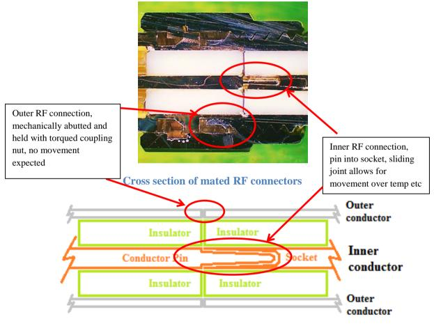
Schematic of mated RF connectors
